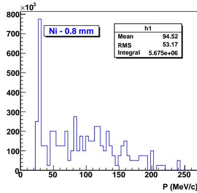
Figure 6: Momentum distribution for muons produced by a 0.8 mm nickel target.
