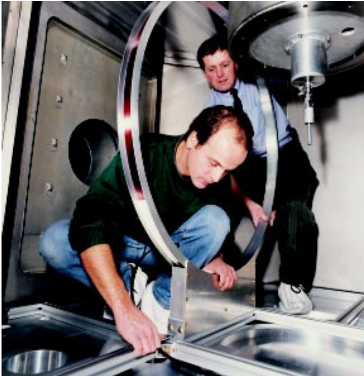
Dennis Abbley and Howard Vizor installing guide field coils on OSIRIS (99RC1109).
