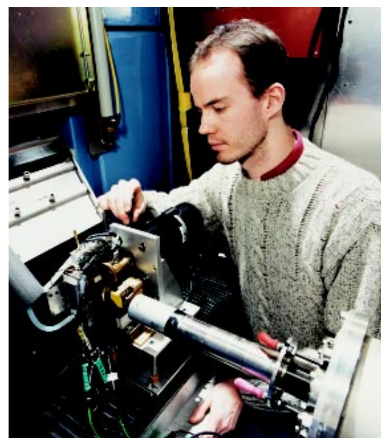
James Holt (Reading University) using the twin plate shear cell, originally developed for SAXS, for the first time on LOQ (99RC5733).
