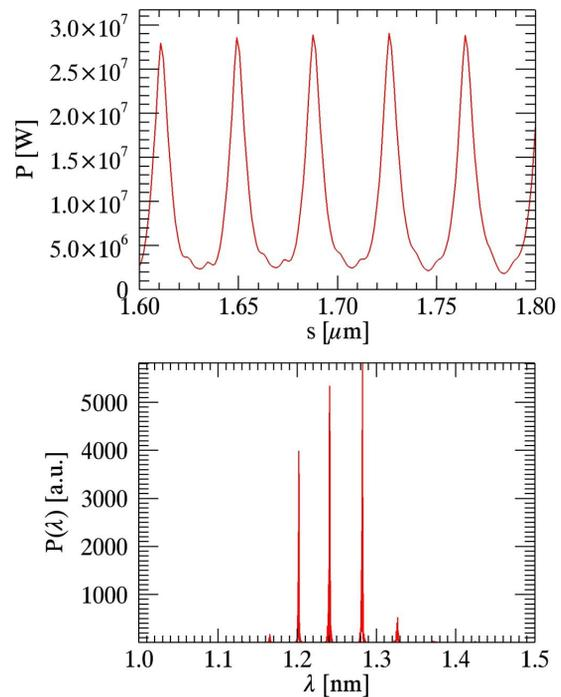
Figure 4: Radiation power profile and spectrum in the radiator after 10 undulator periods.
