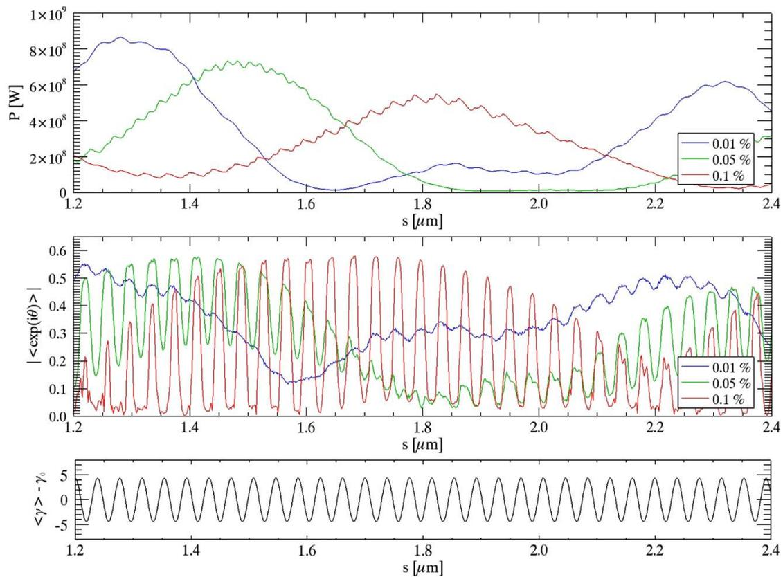
Figure 2: Longitudinal profile of the radiation power (top) and that of the electron beam bunching (middle) are shown for different values of the initial energy modulation amplitude. For each case the plotted data is near to FEL saturation. The beam energy at the entrance to the FEL is shown for the 0.1 % energy modulation case (below), to show the position of the bunching peaks relative to the modulation phase.
