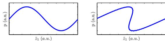
Figure 6: Energy modulation evolution in simulation codes. In the code used, electrons are confined to their initial buckets - density modulation (right) due to an initial sinusoidal modulation (left) is possible on the scale of the radiation wavelength but not on the longer scale of the modulation period.
