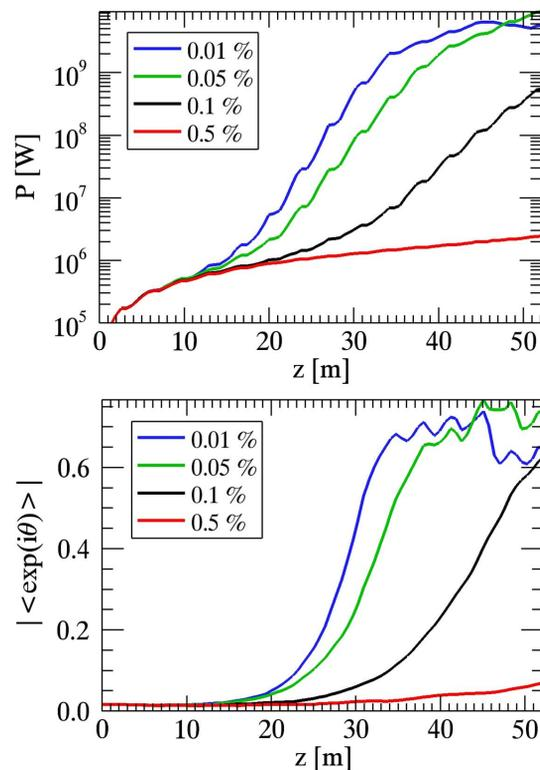
Figure 1: Maximum power (top) and maximum bunching (bottom) in the simulated window plotted against distance through the undulator, for different values of initial energy modulation amplitude.
