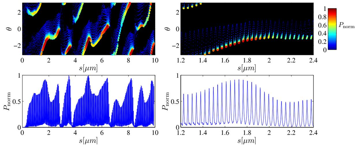
Figure 5: Radiation phase (with plot colour correlated to radiation intensity) and normalised power profile in the radiator after 10 undulator periods, for the simulated 30 fs time window (left), and zoomed to show a 4 fs region (right). The phase is continuous on the scale of a co-operation length.
