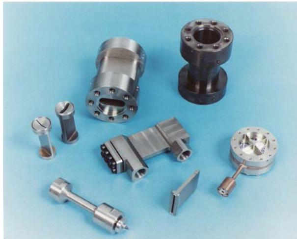
**Fig.1 A view showing a selection of high pressure vessels of differing geometries for neutron use.**
