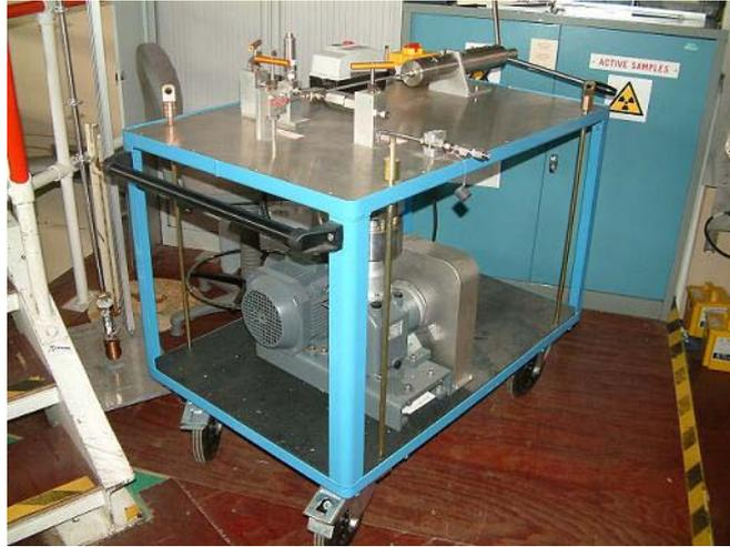
Fig.9 Typical intensifier system mounted inside its mobile trolley assembly.
