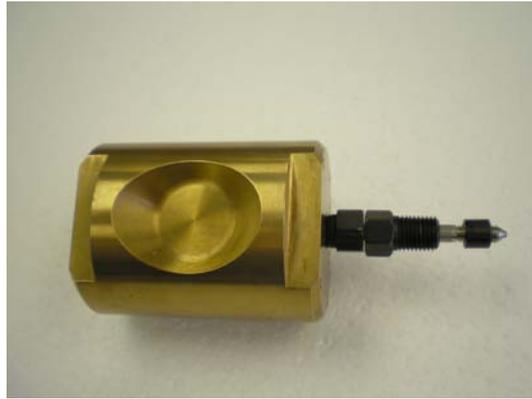
**Fig.2 A beryllium copper high pressure vessel showing a reduced area window.**
