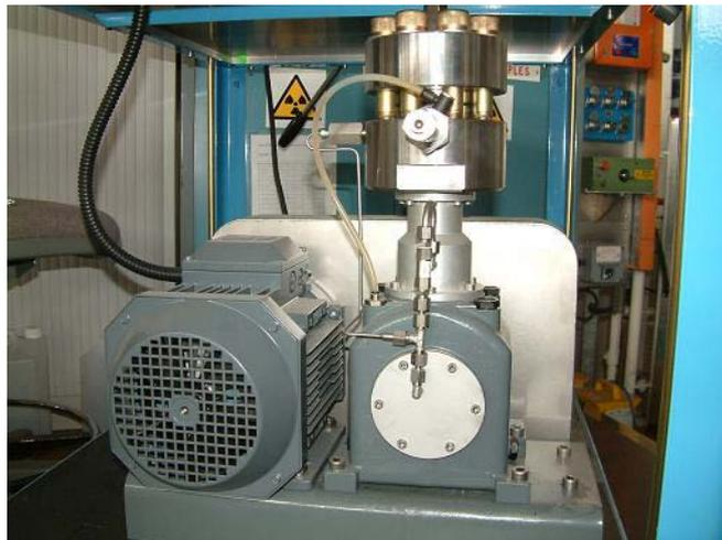
Fig.10 First-stage compressor with its hydraulic oil system at the base and the high pressure gas outlet at the top.
