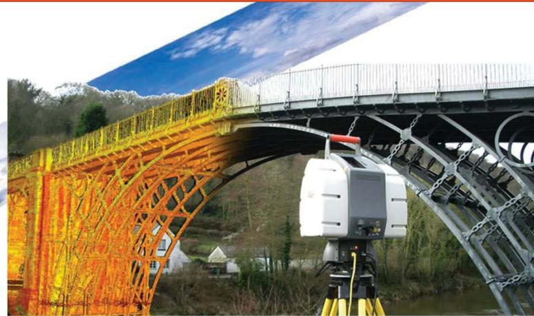
Fig 4. Digital twins of a bridge using 3D scanner
