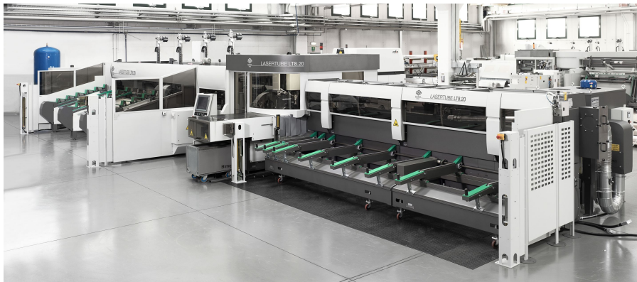
Fig. 1. An Adige LT8 laser machine. These machines cut metal tubes using a cutting head moving along three axes, together with the translatory and rotatory motion of the tube.
