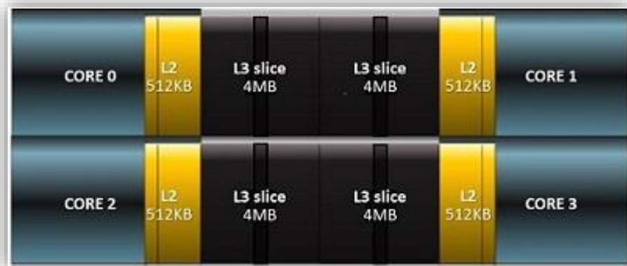
Figure A CCX with four cores and shared 16MB L3 cache
