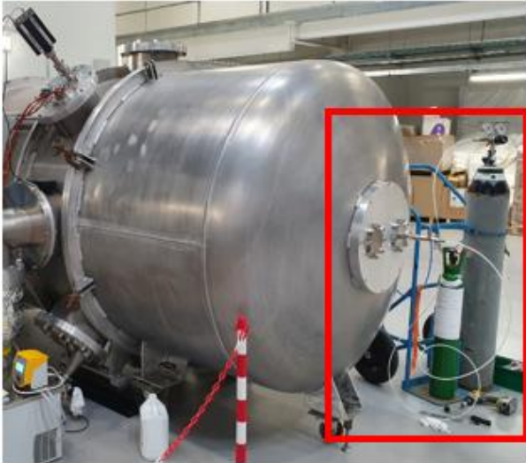
Figure 4: N2 and Ar plus needle valve on inlet. Installed perpendicular to pumping port
