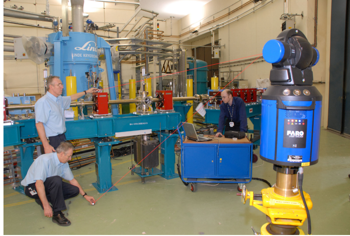
Figure 13.7 Magnets on the ERLP are positioned using the 3D free stationing approach and a laser tracker
