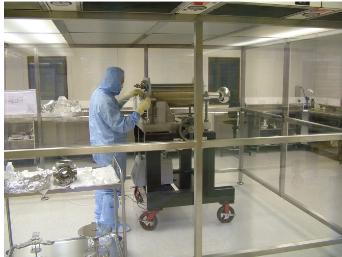
Figure 13.13 ERLP gun being assembled in the ISO class 4 clean room at Daresbury Laboratory
