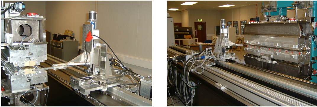
Figure 9.19 Photographs of the HU56 APPLE-II undulator being tested at Daresbury Laboratory
