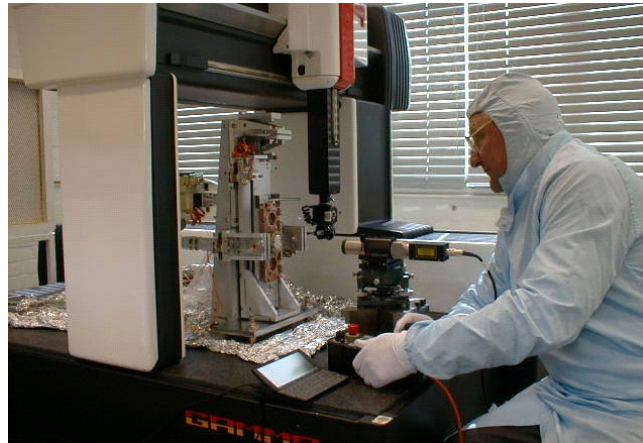
Figure 13.6 A CMM at Daresbury Laboratory measuring the repeatability of the EUFEL optical cavity mirror mechanism
