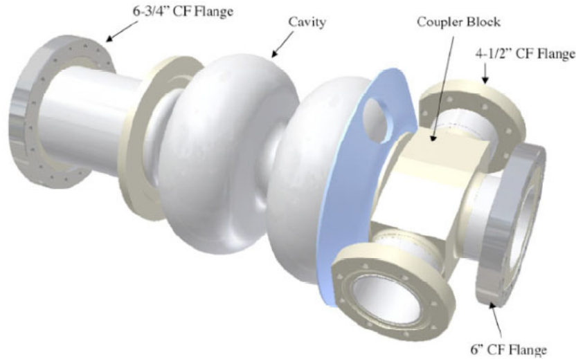
Figure 6.2 Cornell 2-Cell CW injector cavity design (courtesy Cornell University)
