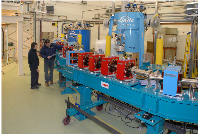
Figure 13.1 ERLP support girder modules installed in the Accelerator Hall
