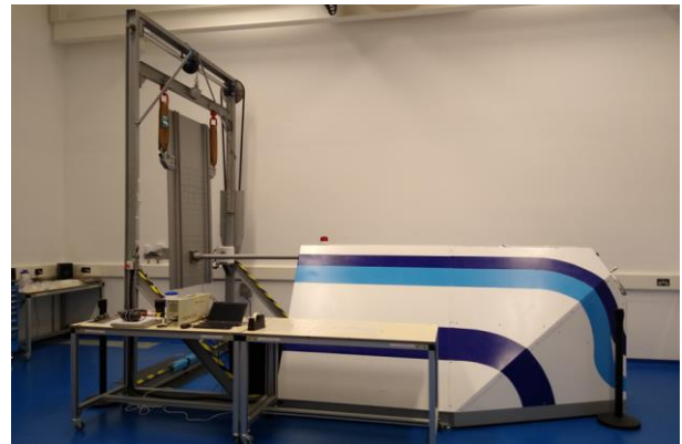
Figure 1: The SERMS Pyroshock Simulator
