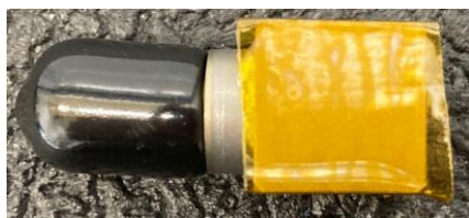
Figure 2: Example of a vibration accelerometer with applied protective tape
