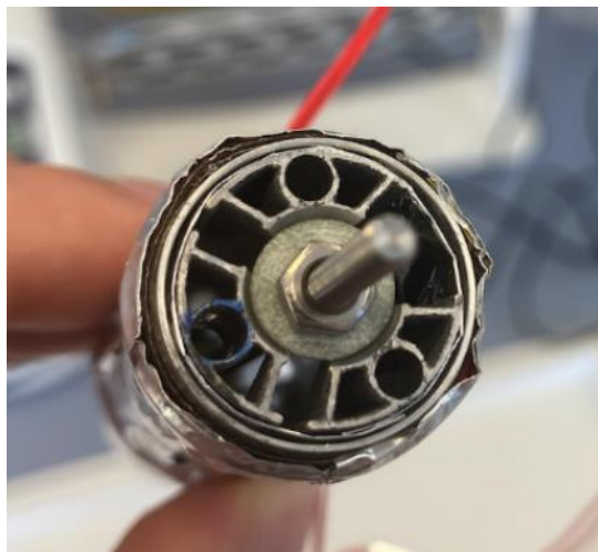
Figure 5: The filled sample sachet placed into the assembled Annular sample can. [3]
