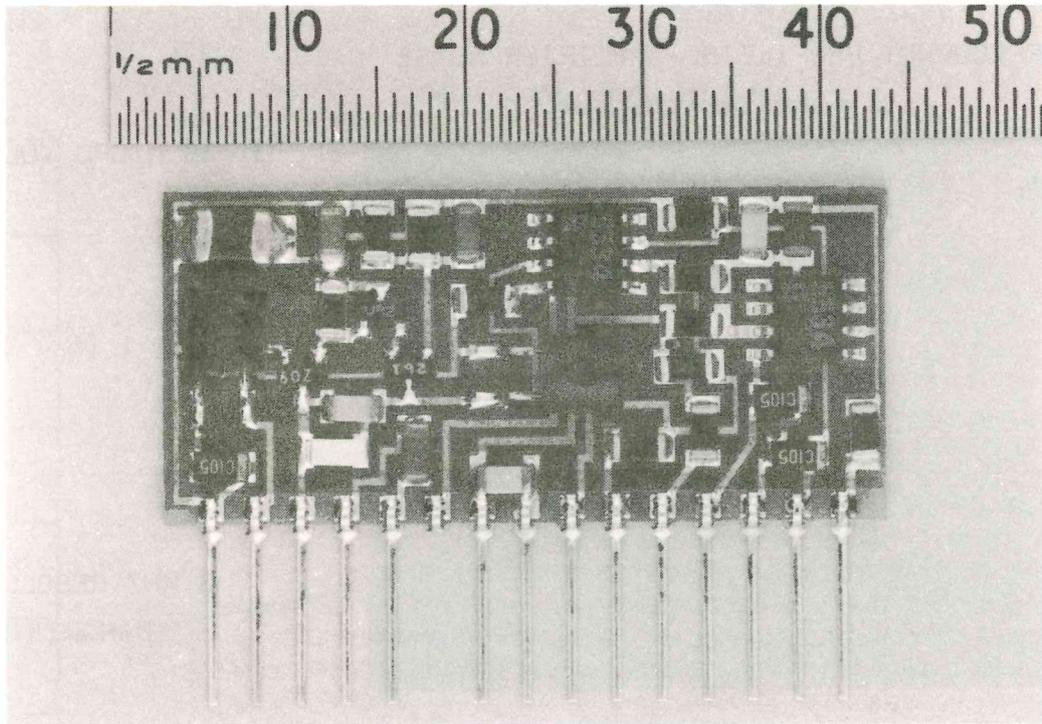
VIEW OF SURFACE MOUNTED PREAMPLIFIER
