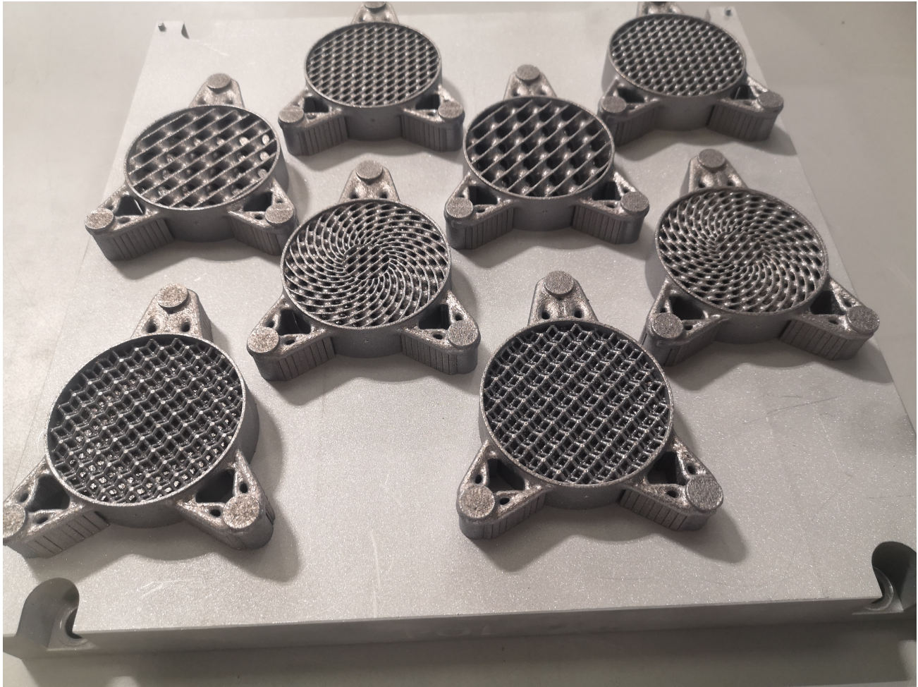
Figure 28: Eight normal resolution parts still on the build plate, support structures can be seen on the mounts. Image credit: Alan Magowan, LPE
