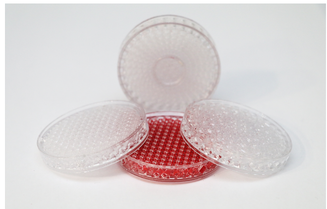
Figure 17: All four lattice tests printed in clear resin, red sand residue is clearly visible in the Fluorite lattice. Image credit: Jason Cowan
