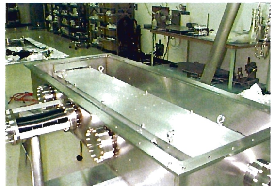
Figure 19: The collimator vessel prior to its installation at SLAC.
