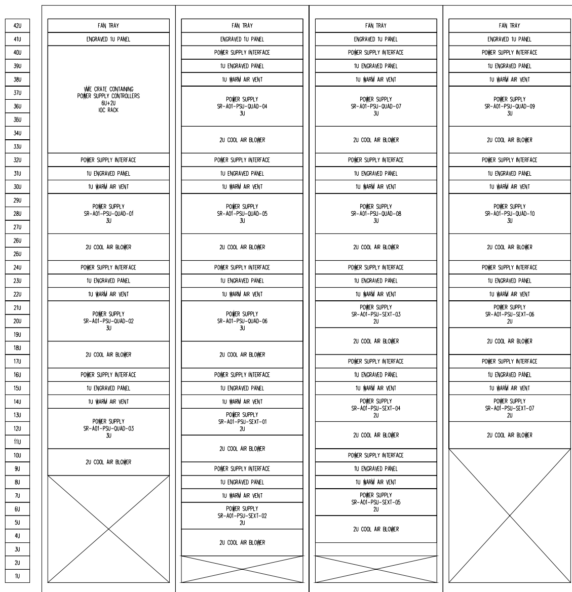
Figure 8.5-1 Arrangement 1 for Quadrupole and Sextupole power converters
