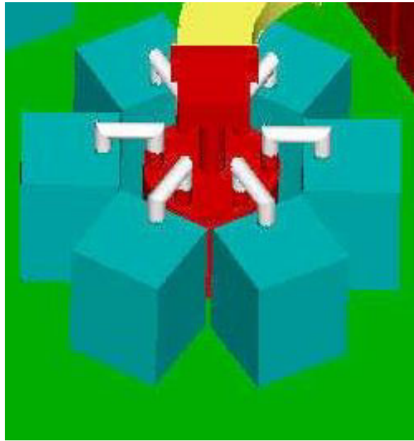
Figure 3.6-2 6 IOTs combined in a combining cavity
