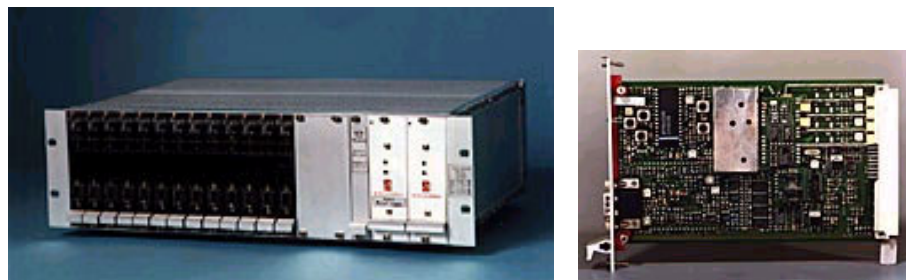
Figure 4.3-1 Bergoz Type Crate For 13 EBPMs, Including Test Station and PSU (individual EBPM card shown also)
