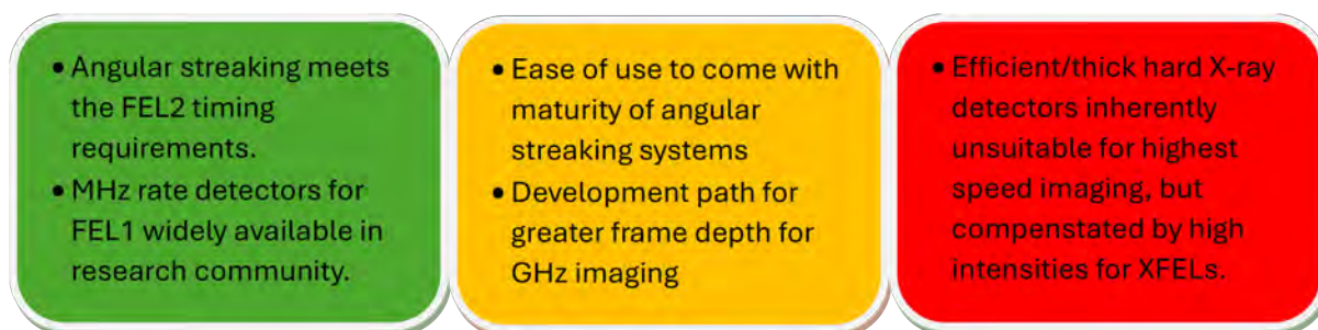
Figure 10.15: Summary of nanosecond and attosecond detector technology.
