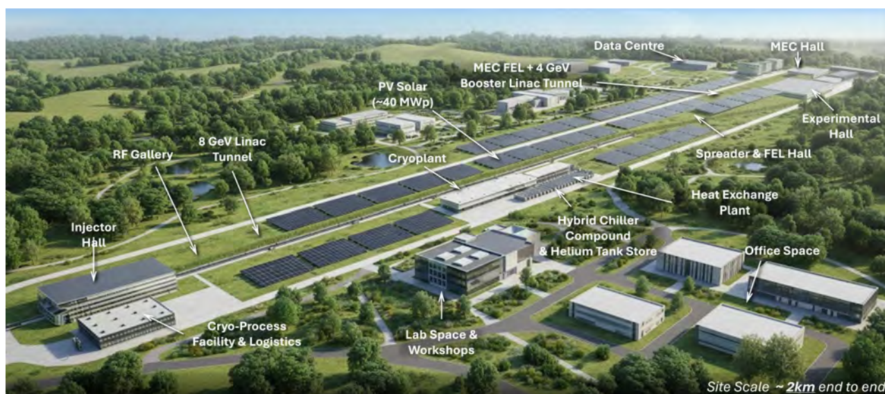
Figure 1.1: Site visualisation of the next-generation XFEL facility.
