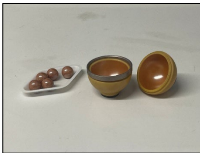
Figure 6. Photo of the \text{ZrO}_2 spherical reactor (15 mL volume capacity) and milling balls (10 mm diameter), as received from the Fritsch company.
