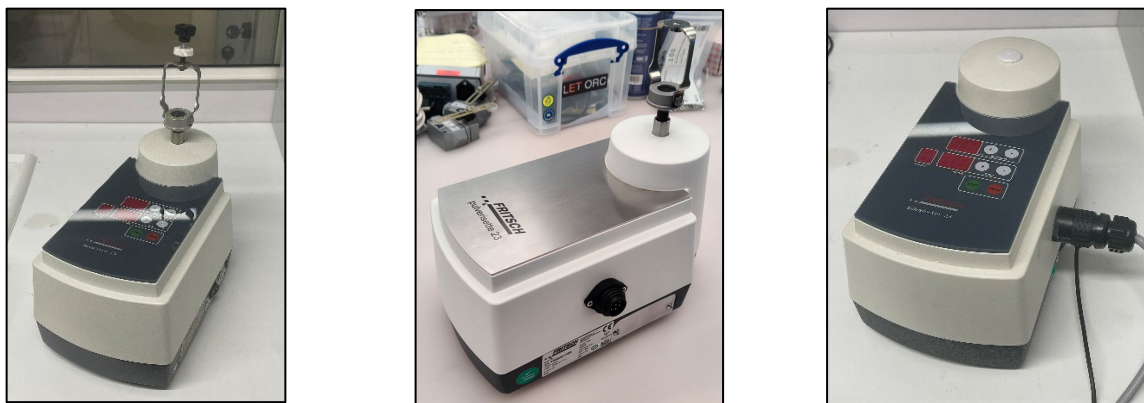
Figure 1. Standard Pulverisette 23 ball-mill (left), and the bespoke version where the ball-mill mechanism (centre) has been detached from the control panel (right).
