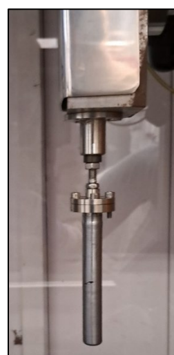
Figure 19. Photograph of the vanadium cans, modified lids and milling balls (8 and 5 mm diameter) (left), insertion of lid in the can (centre), and final assembly attached to ball mill.
