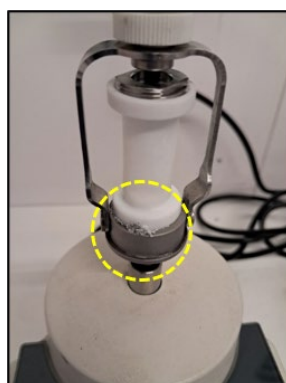
Figure 13. Sample leaking issues (highlighted with yellow dotted circle) encountered with the first PTFE ball mill reactor version.
