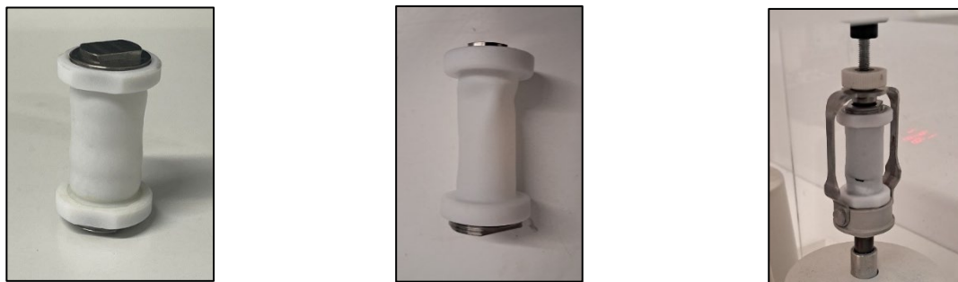
Figure 16. Different instances of the deforming issue encountered after repeated use of the PTFE ball mill reactor.
