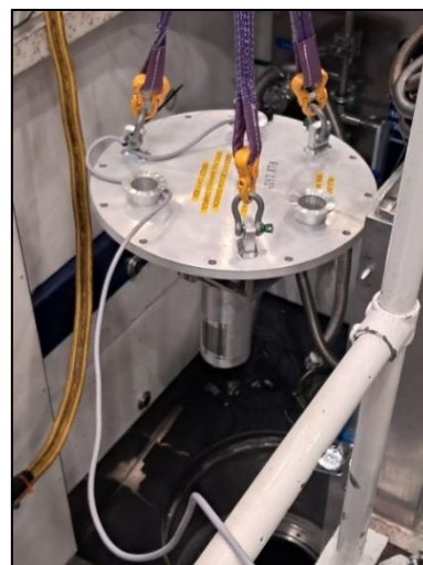
Figure 5. Photographs of the final modified ball mill, sitting on the storage / transportation trolley (left), and being craned from the trolley into the GEM instrument for conducting neutron powder diffraction experiments (centre and right).
