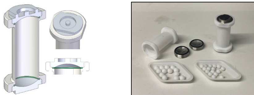
Figure 14. Final design drawings (left) and photo of the PTFE cylindrical reactors (7 mL volume capacity) and milling balls (8 and 5 mm diameter) (right).
