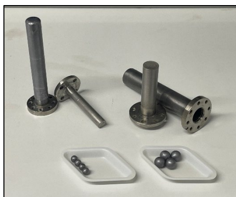
Figure 19. Photograph of the vanadium cans, modified lids and milling balls (8 and 5 mm diameter) (left), insertion of lid in the can (centre), and final assembly attached to ball mill.
