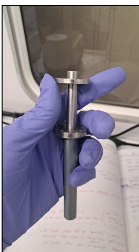
Figure 19. Photograph of the vanadium cans, modified lids and milling balls (8 and 5 mm diameter) (left), insertion of lid in the can (centre), and final assembly attached to ball mill.
