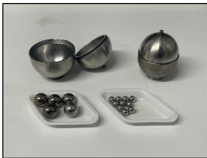
Figure 8. Photo of the stainless-steel spherical reactors (15 and 10 mL volume capacity) and milling balls (10 and 5 mm diameter), as received from the Fritsch company.
