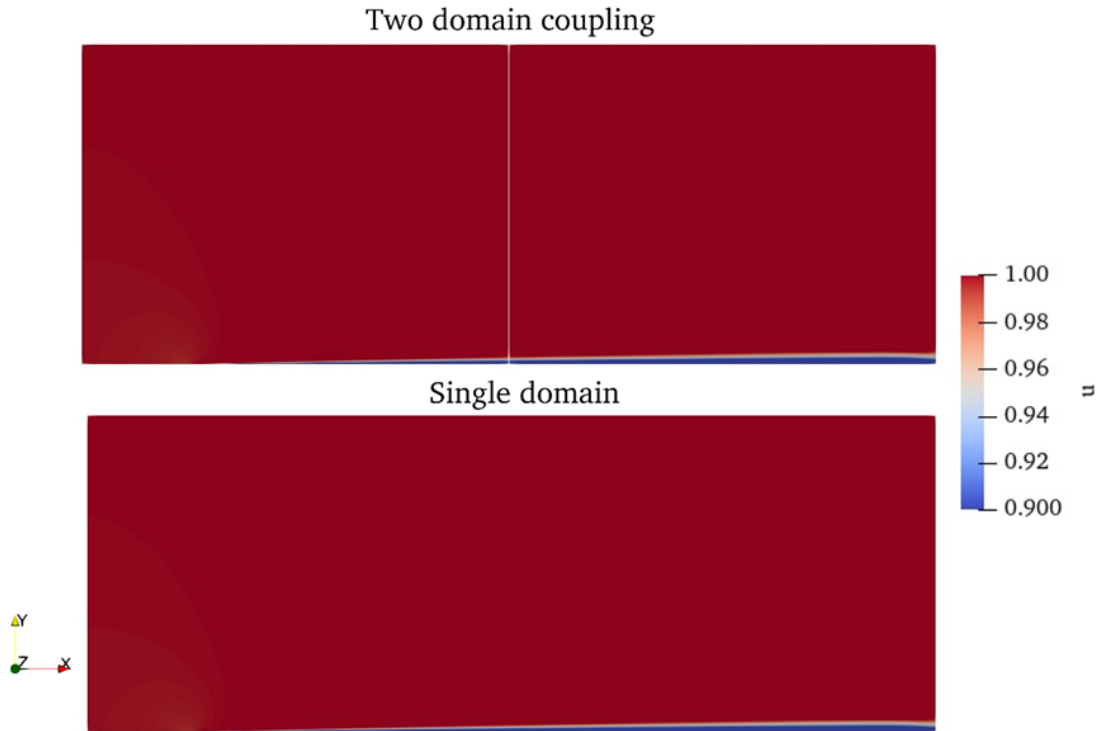
Figure 23 Contour of x -axis velocity ( u ) on two domain coupling (top) and single domain (bottom)
