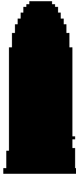
Figure 12: Solution computed on a mesh of 60 \times 60 elements. The buckling constraint is set to c_s = 0.5 and the compliance constraint c_{\max} = 5.5 . In this case, compared with Figure 11, the higher compliance constraint has led to a solution where this constraint is inactive and the buckling constraint is now active.
