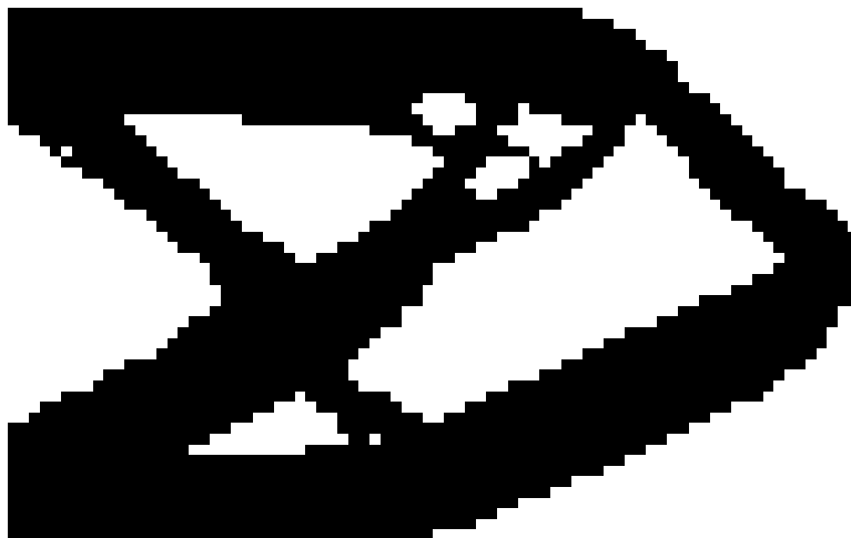
Figure 4: Solution found on mesh of 80 \times 50 elements. The buckling constraint is set to c_s = 0.9 and the compliance constraint c_{\max} = 60 . A volume of 0.5535 is attained. Here the buckling constraint c_2 is active and the compliance constraint c_1 is not.
