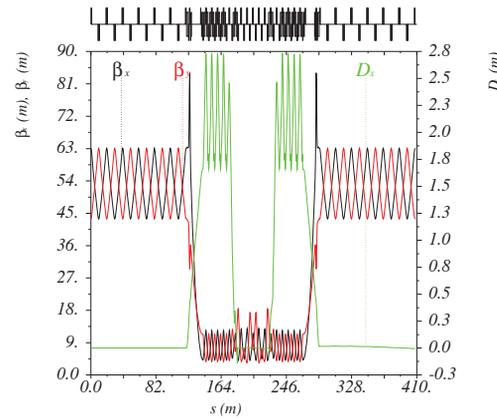
Figure 5: Optics for a preliminary 10 GeV design with an insertion at the centre of the arc and a dispersion suppressor on either side. The suppression of the dispersion can be seen by comparison with Fig. 2.
