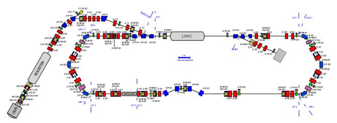
Figure 1: Layout of the ALICE accelerator.
