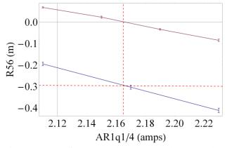
Figure 6:  $R_{56}$  vs. first arc quadrupole strength measured at the exit of the first arc (magenta) and the bunch compressor (blue). The red dotted line indicates the isochronous condition of the first arc.
