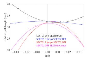
Figure 7: Relative path length vs. energy measured at the exit of the first arc for different arc sextupole (SEXT01 and SEXT02) strengths. Points are measurements, lines are parabolic fits.
