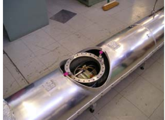
Figure 5: He vessel and magnets inside radiation shields.
