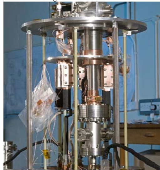
Figure 6: The cryostat turret.
