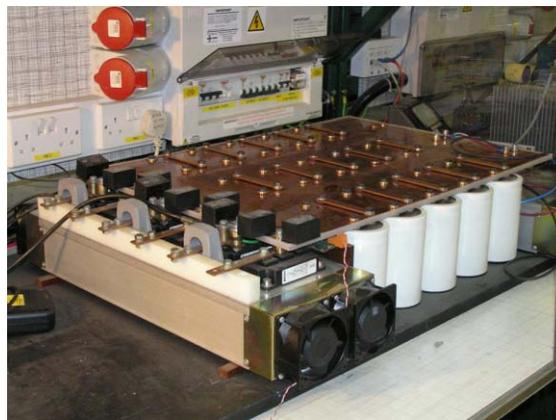
Figure 1: Experimental Multi-Phase Resonant Converter Power Circuit [2,3].
