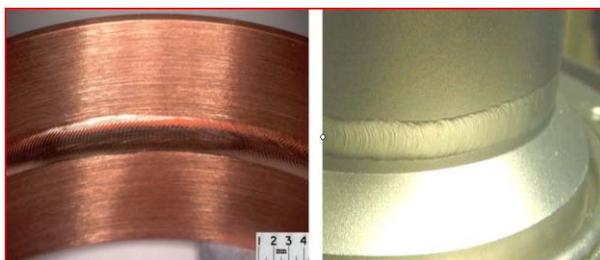
Figure 6: Examples of TIG welding on coupler components. Left: e2v Ltd [3] and right: ACCEL Instruments GmbH [9].
