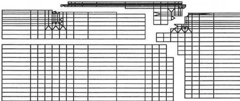
Figure 2: Mesh decomposition of a 2D MOSFET into 4 subdomains.
