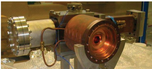
Figure 2: The ALPHA-X S-band RF gun.
