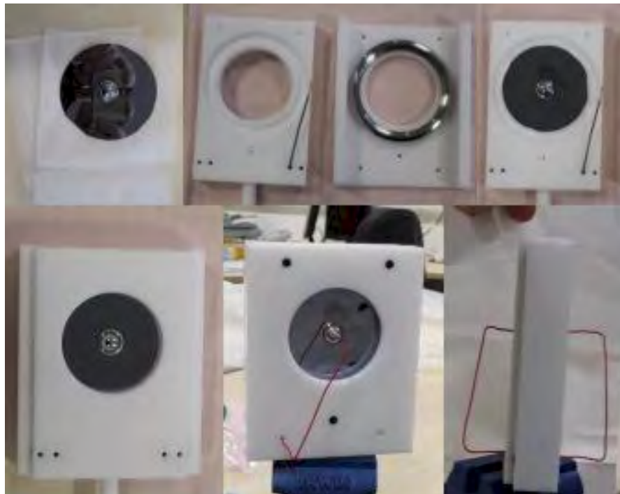
FIGURE 2.19: Stages of antenna assembly
