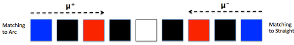
Figure 1: Insertion section schematic. The black rectangle represent triplet magnets while the red and blue rectangles represent kicker magnets and septa, respectively. The empty long drift is shown as a white rectangle.
