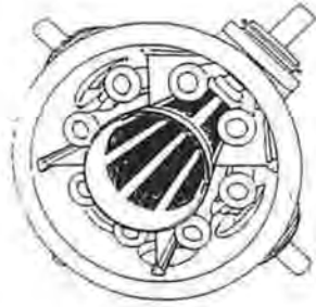
Figure 7: Cut-away view of the Titania diode and laser vessels. Mid-plane current returns removed for clarity.
