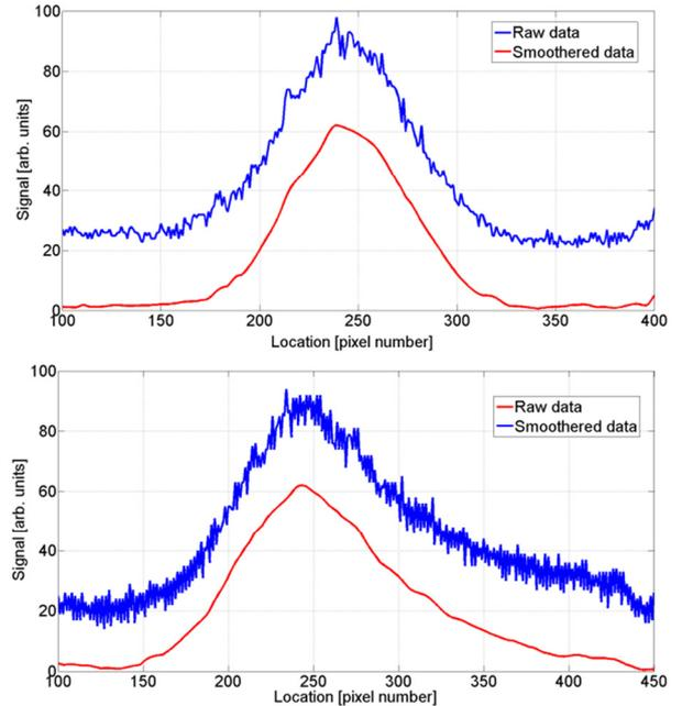
Figure 3: Beam profiles in raw format and smoothed by MATLAB ‘smoothn’ algorithm [6] in the horizontal (upper) and vertical (lower) planes.
