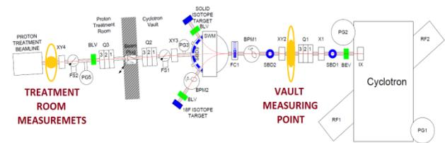
Figure 1: CCC treatment beam line outline. Q1, Q2, Q3 – consecutive quadrupole triplets, X, XY – horizontal or horizontal and vertical steering magnets, SW – switching dipole magnet, yellow marks – quadrupole scan experimental places.
